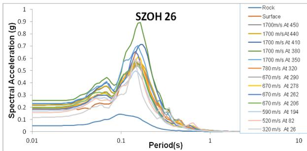
Figure 9. Variation of PSA for site SZOH26 for layers at different depths and corresponding shear wave velocities.
