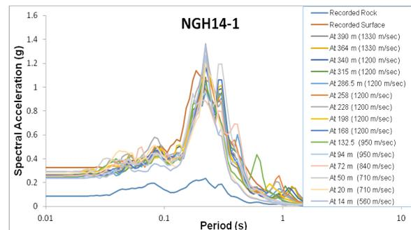
Figure 7. Variation of PSA for site NGH14-1 for layers at different depths and corresponding shear wave velocities.
