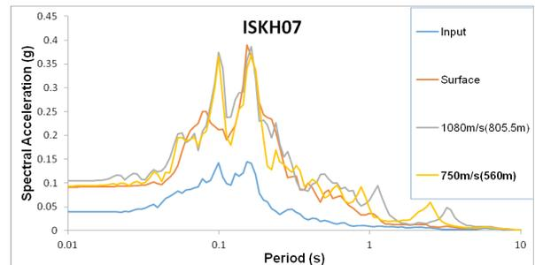
Figure 6. Variation of response spectra for profile ISKH07 showing only matched response to surface response.
