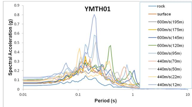
Figure 11. Variation of PSA for site YMTH01 for layers at different depths and corresponding shear wave velocities.
