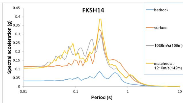
Figure 14. Variation of response spectra for profile FKSH14 showing matched response to surface response.
