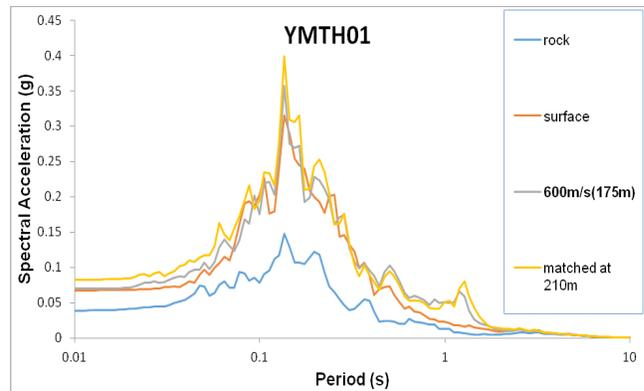
Figure 12. Variation of response spectra for profile YMTH01 showing matched response with surface response.
