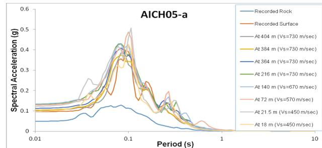
**Figure 1.** Variation of PSA for site AICH05 – for layers at different depth and corresponding shear wave velocities.
