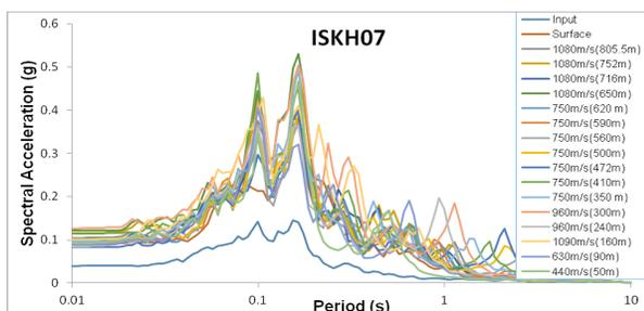
Figure 5. Variation of PSA for site ISKH07 for layers at different depths and corresponding shear wave velocities.
