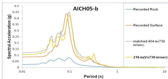
Figure 4. Variation of response spectra for profile AICH05-b showing matched response to surface response.
