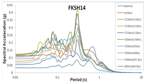
Figure 13. Variation of PSA for site FKSH14 for layers at different depths and corresponding shear wave velocities.
