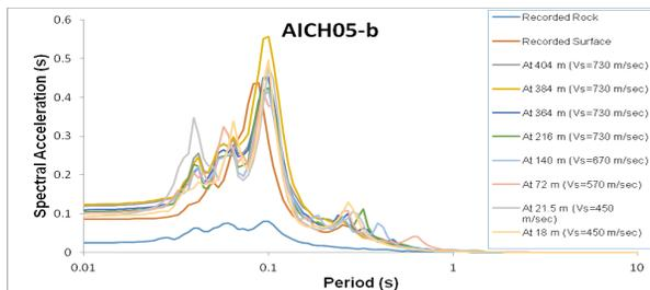
Figure 3. Variation of PSA for site AICH05-b for layers at different depths and corresponding shear wave velocities.
