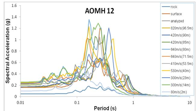
Figure 15. Variation of PSA for site AOMH12 for layers at different depths and corresponding shear wave velocities.
