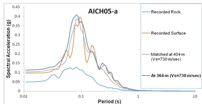
**Figure 2.** Variation of response spectra for profile AICH05-a showing matched response to surface response.
